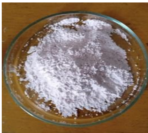
Figure 4 HAp Powder from Anadara Granosa Shells.
