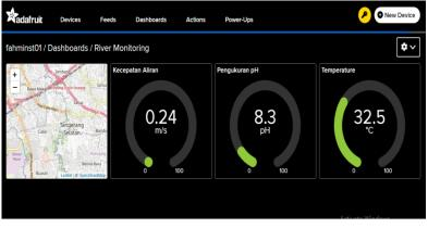
Figure 12 Display of Buoy to Cloud Measurement Results
