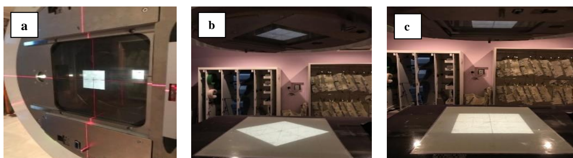
Figure 2 The process of testing the quality control of mechanical in the Department of Radiotherapy at Pasar Minggu District Hospital: Laser testing (a), Collimator testing 45° C (b), Light Field Size testing 10x10 cm 2 (c).
