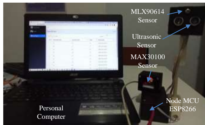
Figure 9. The overall design of heart rate, oxygen saturation, and temperature monitoring system.
